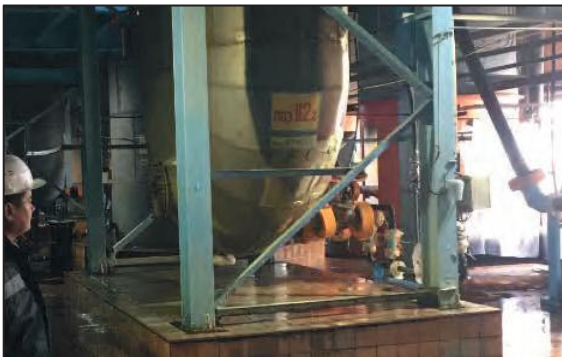
Figure 10-7: Innovative U-shaped column used to improve grade in ion exchange step. Central Moinkum
