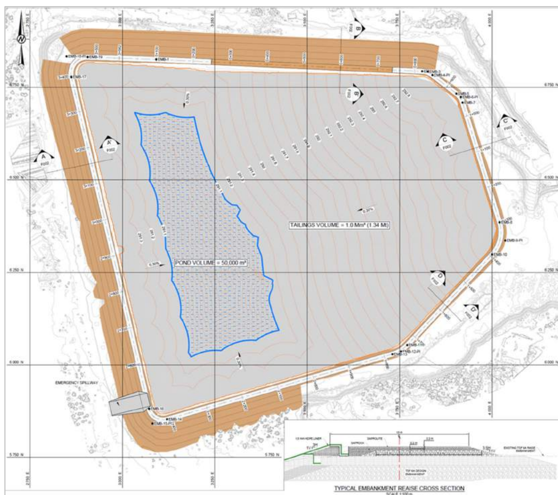
Figure 11-17: Taparko TSF General Arrangement Final Raise
