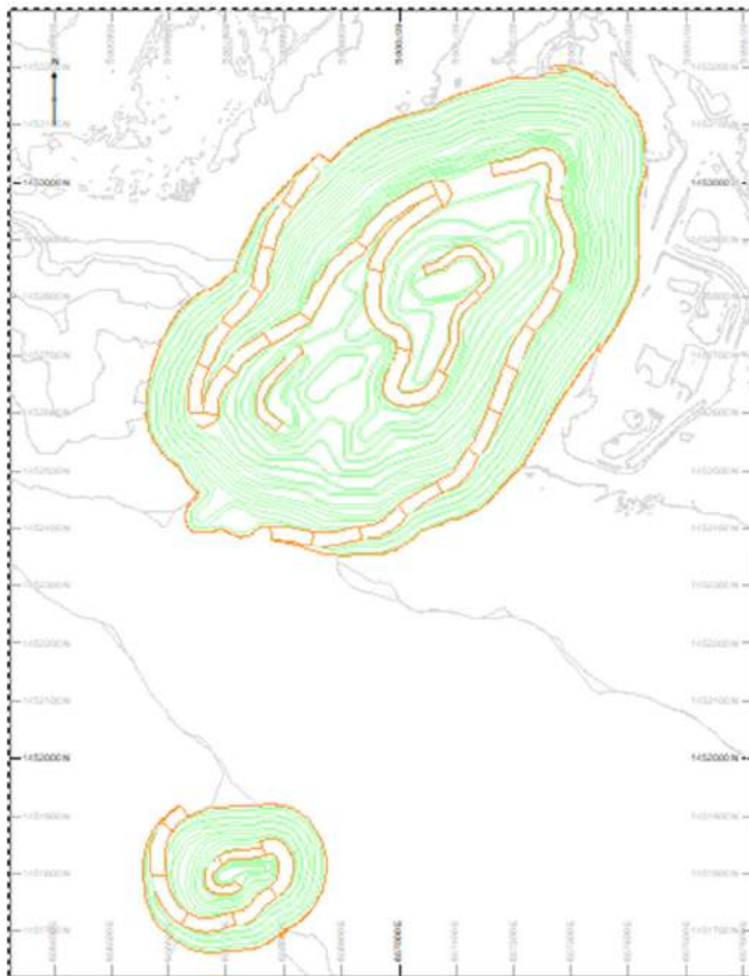
Figure 10-9: Zandkom Pushback 3 and 6 Pit Design (Nordgold 2021)
