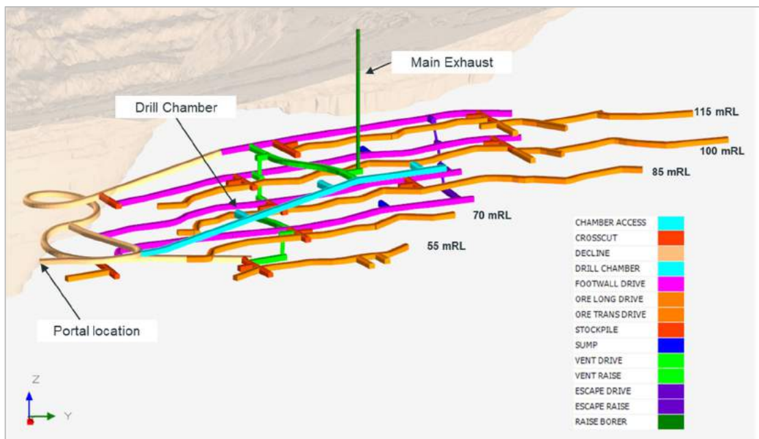
Figure 11-8: Taparko Underground Ore Reserve Case Development Design
